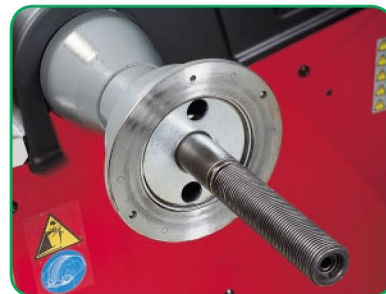
Quick clamping with preloaded spring mounted inside the bell
