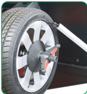
Automatic outside sensor for width measurement
